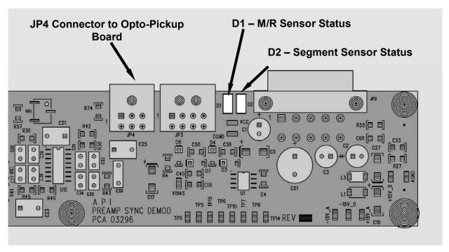
**Figure 12-4:** Sync/Demod Board Status LED Locations
